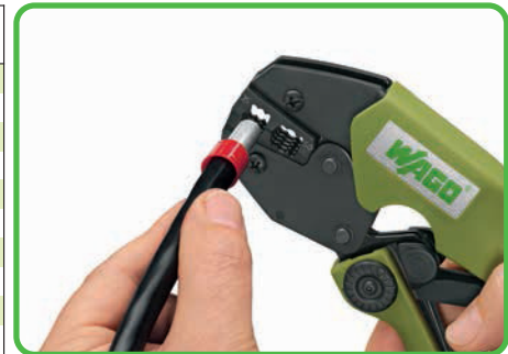
Insert ferruled conductor into crimping station.
