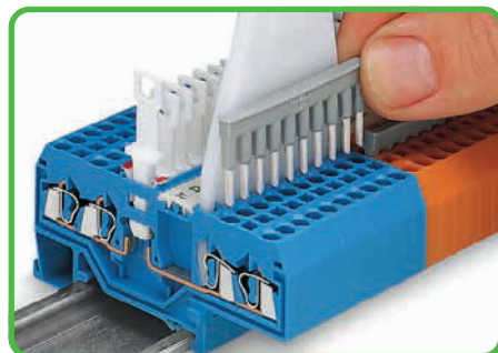
Commoning front-entry disconnect terminal blocks with comb-style jumper bars via 10-way operating tool.
