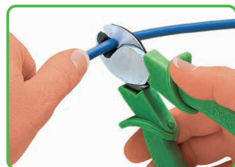
Cutting a conductor.
