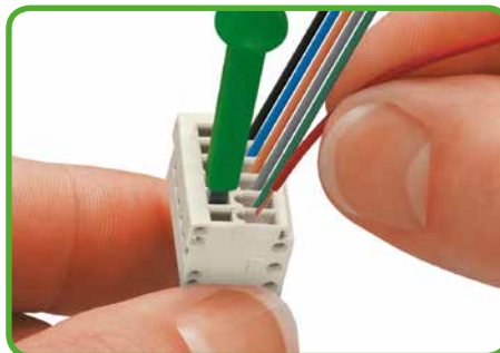
Inserting conductor via 233-335 operating tool. Operation parallel to conductor entry.
