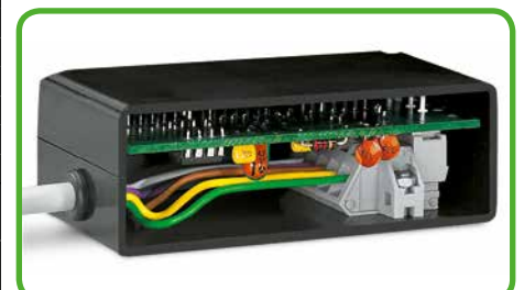
Angled female connector mounted within a housing. A male header with straight solder pins is used for horizontal PCB mounting in narrow housings.
