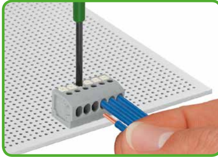
Inserting solid conductor via push-in termination. Inserting and removing fine-stranded conductors via push-buttons.
