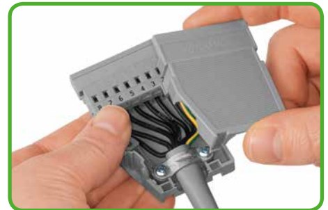
Snapping on a strain relief housing, demonstrated with a male connector. Cable exits laterally. Strain relief by cable clamp.
