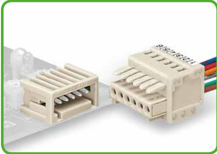
Male header and female connector – 100% protected against mismatching. Only mating halves with the same pole number can be connected together.
