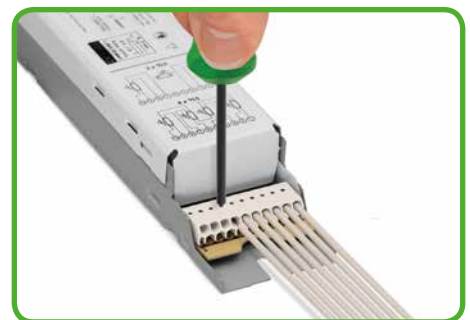
Removing conductor via 1.0 mm Ø disconnection tool. (206-840)
