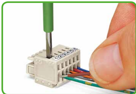
Inserting conductor via (2.5 x 0.4) mm screwdriver. Actuation perpendicular to conductor termination.
