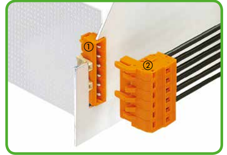
① Male header, angled solder pins ② Angled female connector, conductor entry opposite of latches
