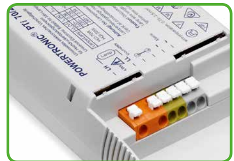
804 Series Terminal Strips provide "internal commoning" to meet requirements for not routing the ground (earth) conductor over the board. This enables custom terminal strips to be commoned and marked at the factory upon request.
