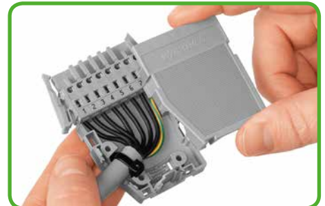
Snapping on the strain relief housing, demonstrated with a female connector with locking levers. Cable exits laterally. Strain relief by cable tie (up to a width of 4 mm).
