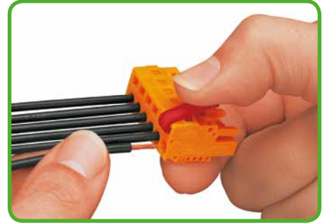
Inserting conductor into CAGE CLAMP® unit via 231-291 operating lever.
