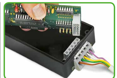
Angled female connector used as through-panel connector. Termination ports and operating slots are located outside the housing. Panel thickness up to 2 mm/0.079 in. Picture shows 5 mm pin spacing.
