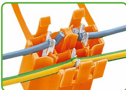
Snapping socket halves together will automatically cut and terminate a "live" conductor without stripping, allowing switching applications (e.g., door switches).
