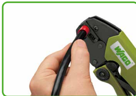
Squeeze handles until ratchet mechanism is released.
