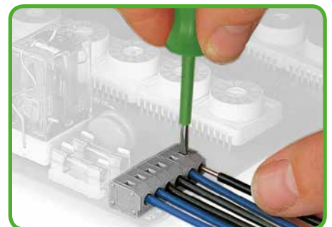
Conductor removal via screwdriver (2.5 mm x 0.4 mm)
