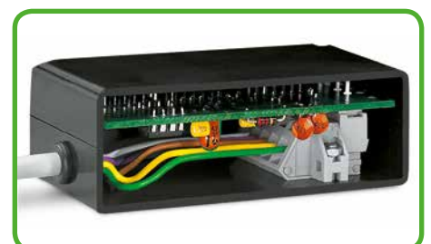
Angled female connector mounted within a housing. A male header with straight solder pins is used for horizontal PCB mounting in narrow housings.
