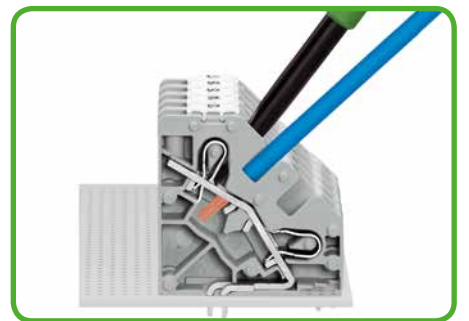
Inserting fine-stranded conductors via 5.5 mm screwdriver.
