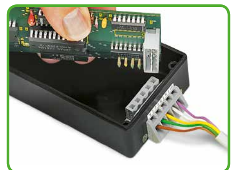
Angled female connector used as through-panel connector. Termination ports and operating slots are located outside the housing. Panel thickness up to 2 mm/0.079 in.
