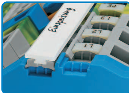
Carrier for WFB Continuous marking strip; to be secured into every 10th terminal block.
