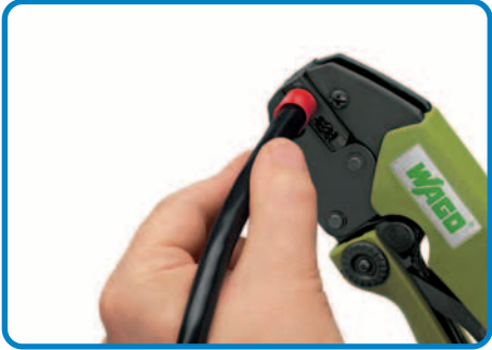
Squeeze handles until ratchet mechanism is released.
