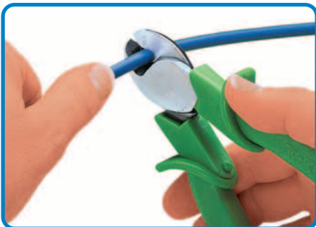
Cutting a conductor.
