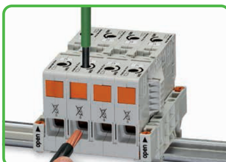
Conductor termination: Insert stripped conductor until it hits backstop; hold this in position.
