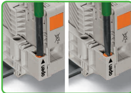
Fixing the assembly: Turn the latch on the mounting adapters from the open to the closed position using an operating tool.
