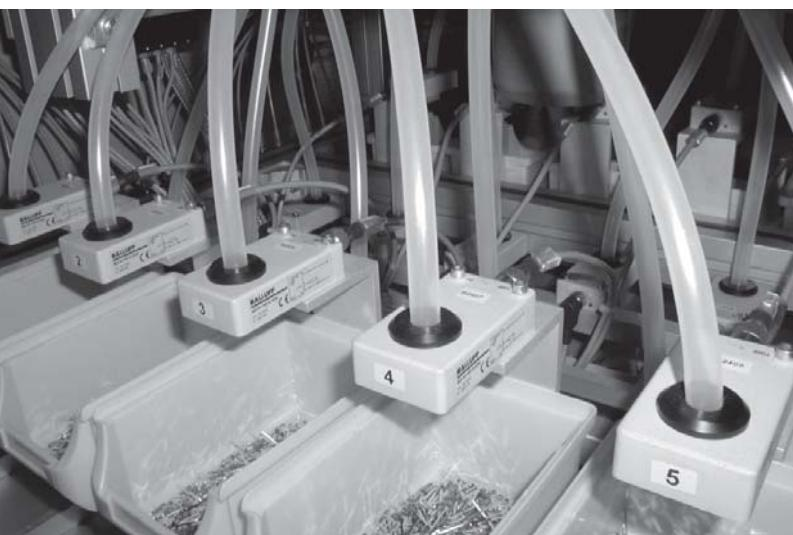
Ring sensors are used for feed control with screws, nails etc.
