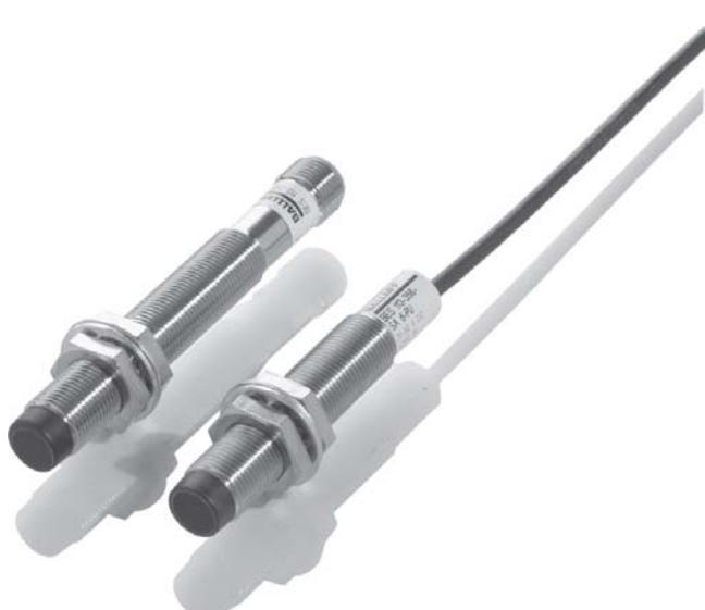
The function diagnostics unit BES 113-FD-1 monitors a proximity switch and its cable using dynamic function diagnostics. A logic circuit polls the sensor signals for the presence of test pulses and also monitors for proper function of the processor. For the machine controller it emits a High level signal on the "Status/Output" line when there is no fault and a Low signal when a fault is present. LED's indicate the switching state of the sensor.
