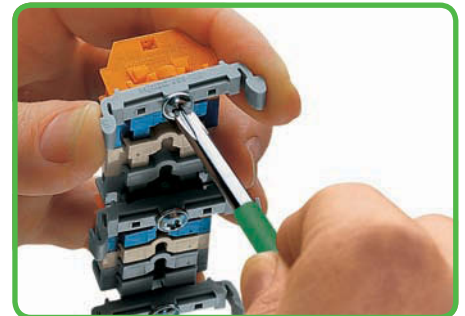
Terminal strip with fixing flanges, screw mounting of 209-123 mounting adapter (distance between mounting adapters should be 35-40 mm).
