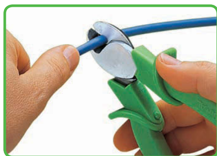
Cutting a cable.
